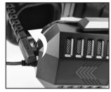
Secure the Microphone by Rotating it 90 Degrees Counterclockwise
